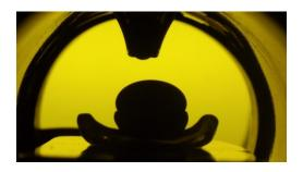
Fig. 2 – A picture of a drop of fusion of Sn + 0,1%In on a quartz cup
